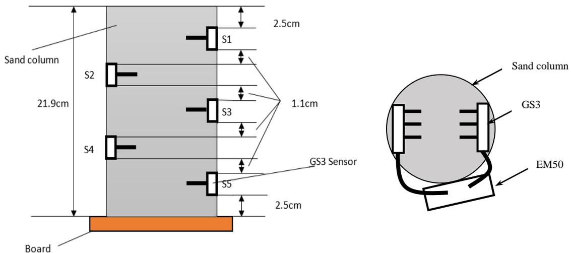
Fig. 2 - Cross-section side (left) and top (right) view of the sand column designed. The S1 to S5 are the soil moisture sensor (GS3). Note that the inner diameter of the column was 21.9 cm.
