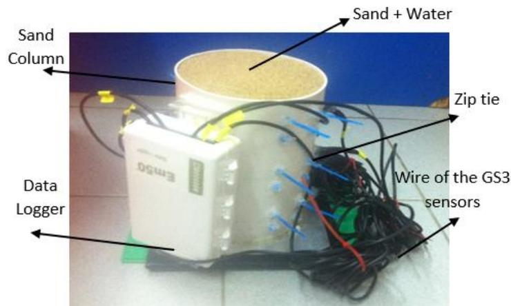
**Fig. 3 - Vertical sand column**
