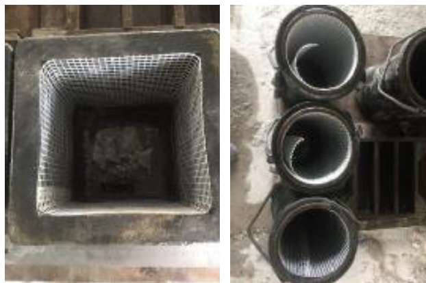
Fig. 3 - The fiber mesh was cut and laid according to the dimensions of the moulds
