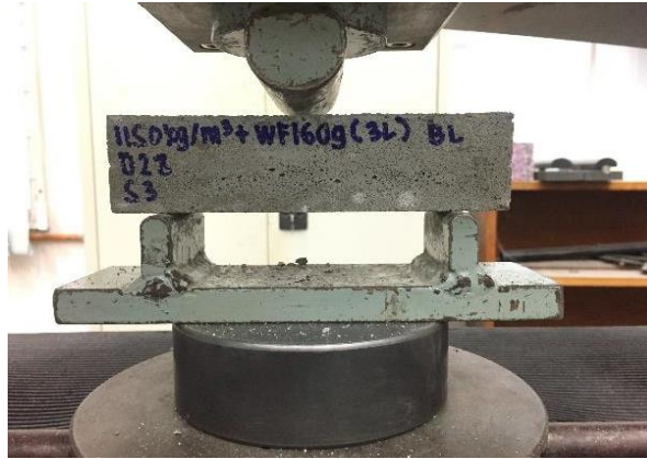
Fig. 7 – Test for load-carrying capacity in bending.
