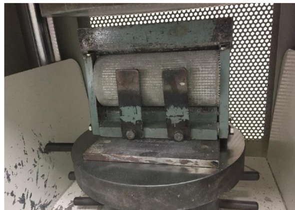
Fig. 8 - Test load-carrying capacity in tension
