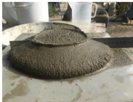
Fig. 4 - Slump test of LFC mix
