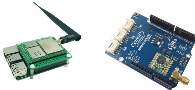
Fig. 1 - (a) LoRa Gateway; (b) LoRa Node
