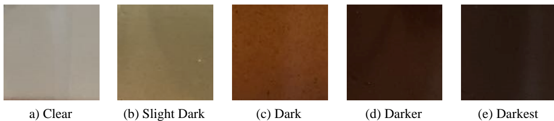
Fig. 7 - Samples of water clarity to validate the turbidity sensors inside the laboratory
