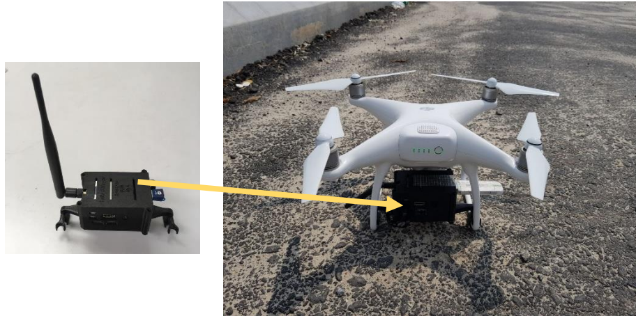
Fig. 12 - Visualisation of Drone-LoRa enable on multirotor drone
