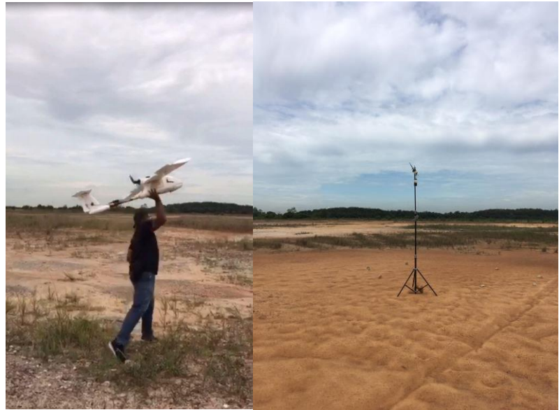
Fig. 20 - A fixed-wing drone and a LoRa gateway involved during the performance measurement
