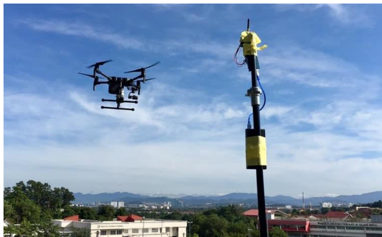
Fig. 13 - Drone-LoRa enable and LoRa on 2 meters tripod
