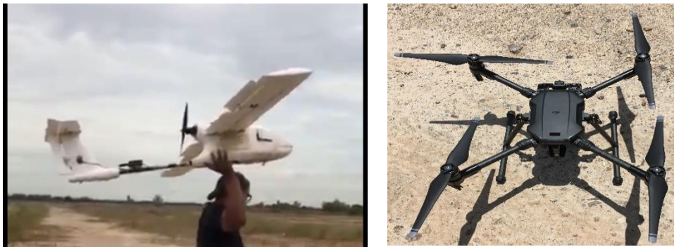
Fig. 2 - (a) Skywalker Fixed-Wing; (b) M200 Multirotor
