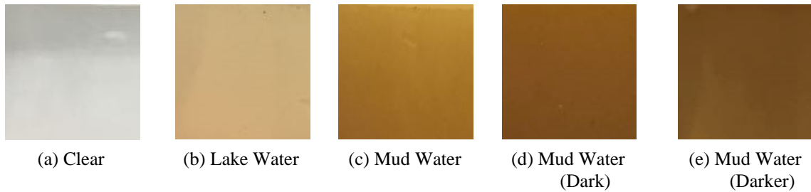
Fig. 9 - Samples were taken from the actual water lake to validate the turbidity sensors
