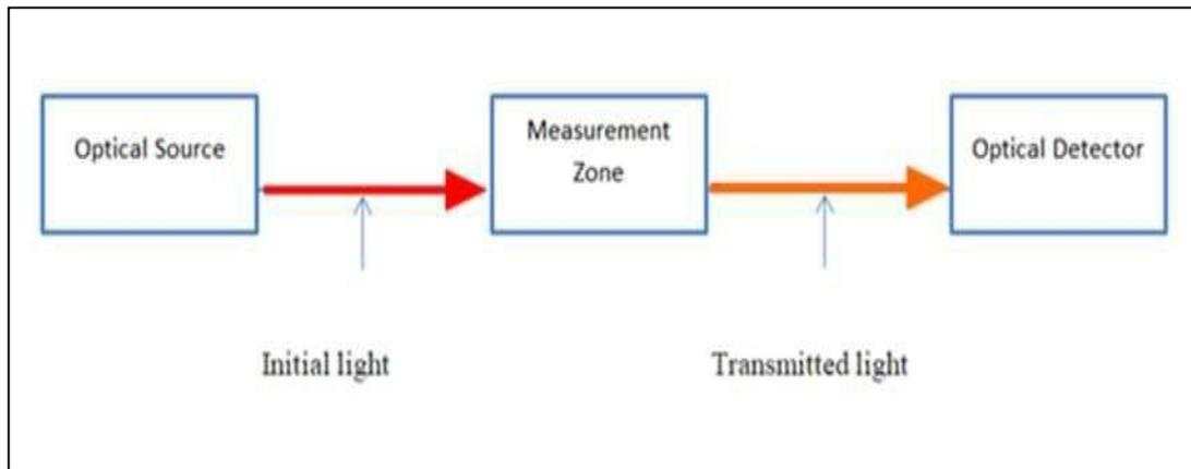
Fig. 2 - Basic working principle of optical sensor
