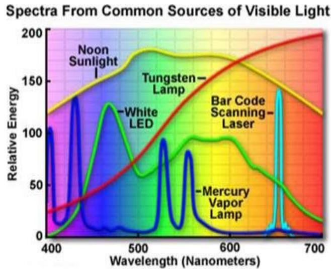
Fig. 1 - Relative energy vs. wavelength for spectra from common sources of visible light
