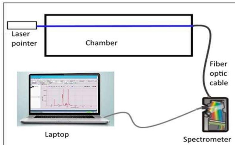
**Fig. 4 - Experimental setup for laser stability test**
