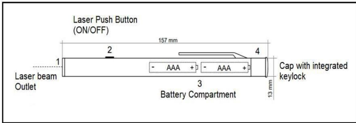
**Fig. 3 - Schematic diagram of a laser pointer**
