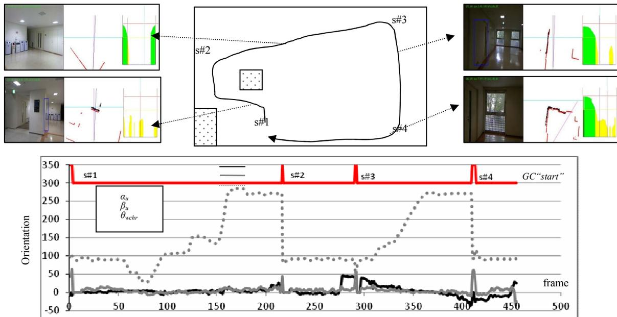
Figure 5: GC in hallway navigation. (Top) Illustration of maneuvering path with sample snapshot. (bottom) Command state transition and its effect to overall maneuvering direction.
