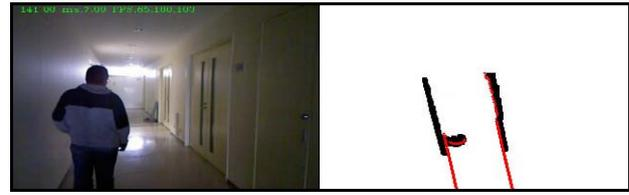
Figure 3: RGB image (left) and Navigation map image (right). Black areas and red areas sourced from Kinect and laser sensor respectively.
