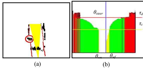
Figure 4: Sample of navigation map for Figure 3. (a) The black area source from Kinect, laser area is denoted by red color and yellow area indicates free spaces. (b) Visualization of the generated POD
