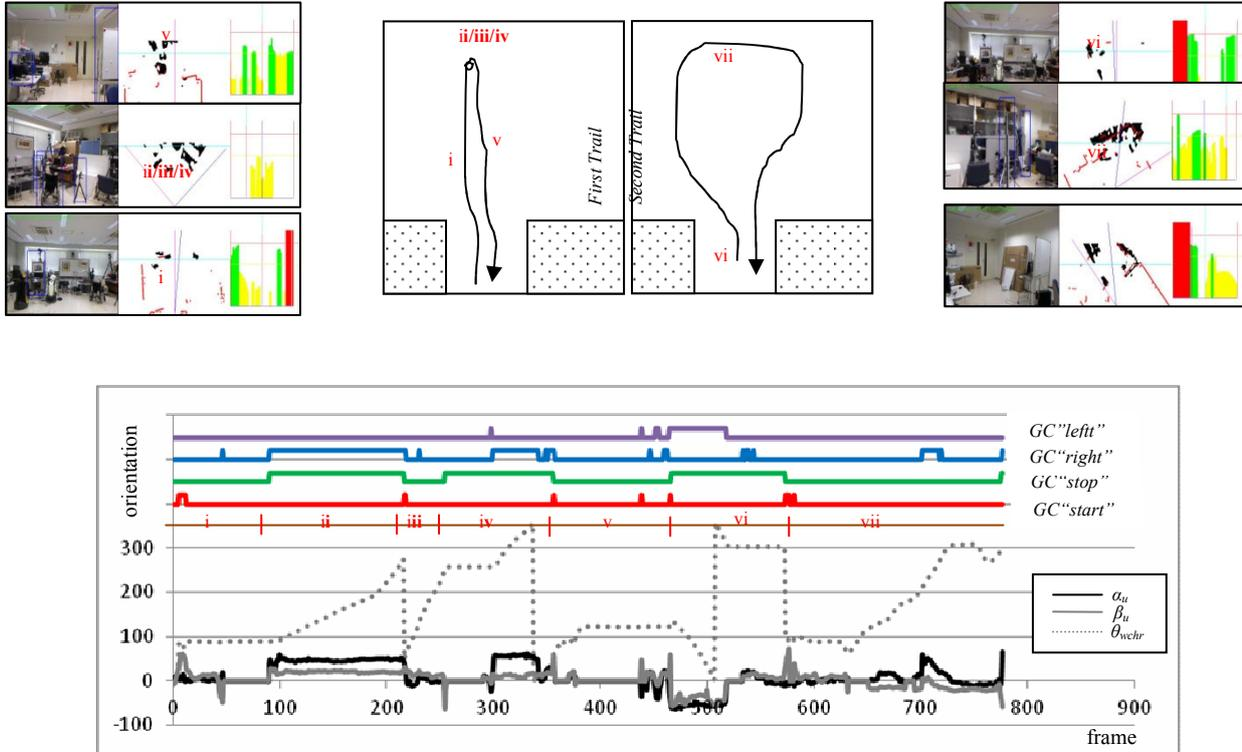
Figure 6: GC in lab navigation. (Top) Illustration of maneuvering path with sample snapshot. (bottom) Command state transition and its effect to overall maneuvering direction.
