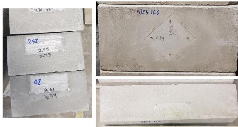
Fig. 1 - locations of strain discs on the specimen
