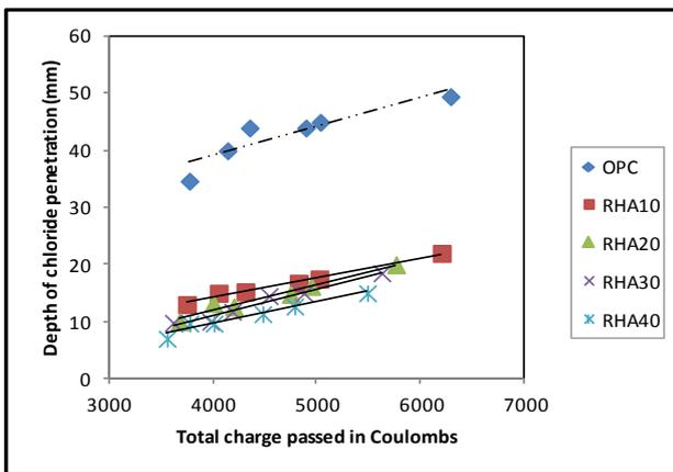
Fig. 2 Relationship between total charge passed and depth of chloride penetration.
