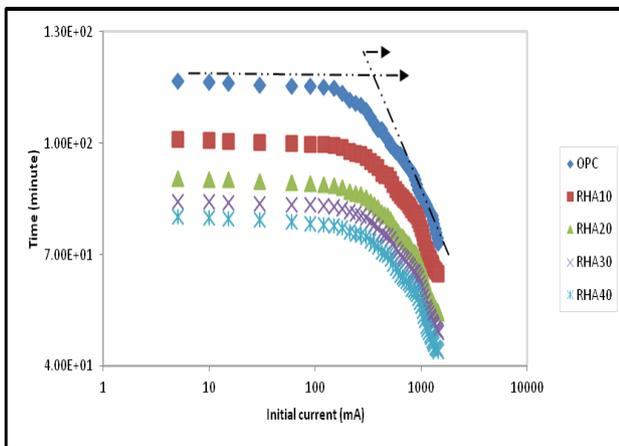
Fig. 4 Graphical determinations of primary and secondary slopes for OPC and RHA blended cement concrete.
