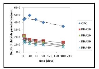
Fig. 1 Depths of chloride penetration of specimens under seawater attack with wetting-drying cyclic
