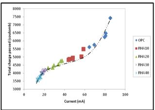
Fig. 3 Relationship between total charges passed and initial current for OPC and RHA blended cement concrete.
