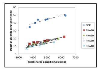
Fig. 2 Relationship between total charge passed and depth of chloride penetration.
