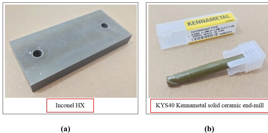
Fig. 1 - Specimen and cutting tool (a) Inconel HX; (b) KYS40 Kennametal solid ceramic end-mill
