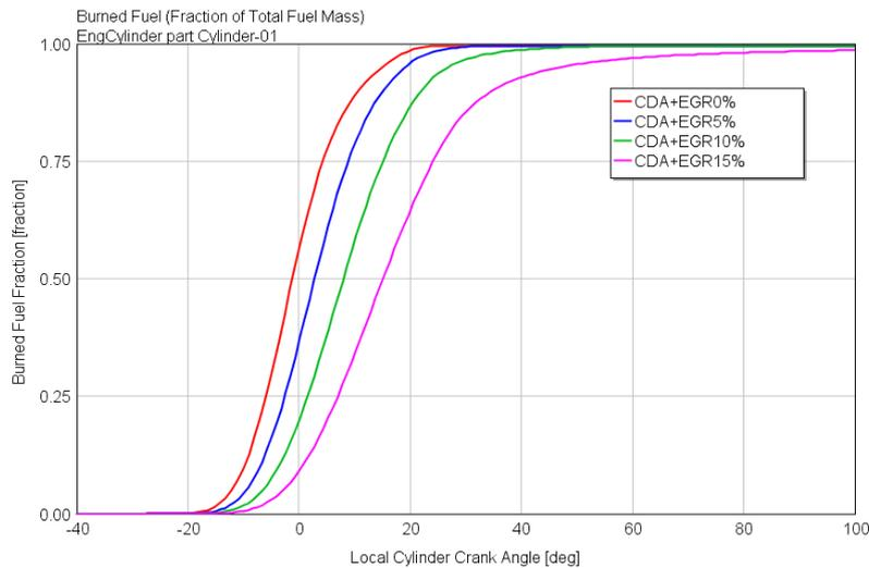
**Fig. 12 - Burned fuel fraction for different percentages of EGR at 2000rpm@3bar BMEP**
