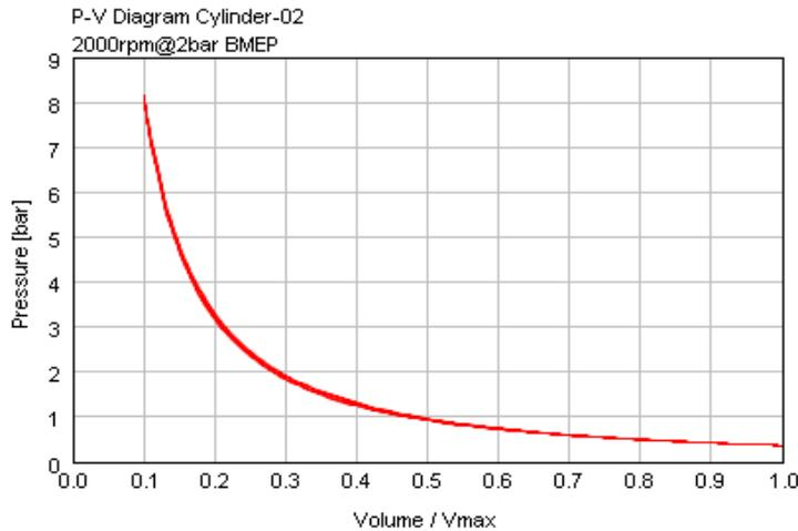
**Fig. 7 - Predicted cylinder pressure of an unfired cylinder at 2000 rpm, 2 bar BMEP**
