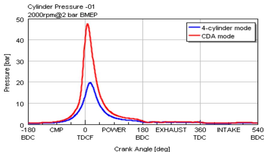
Fig. 5 - Predicted combustion pressure for normal 4-cylinder mode and CDA mode operations at 2000 rpm@2bar BMEP
