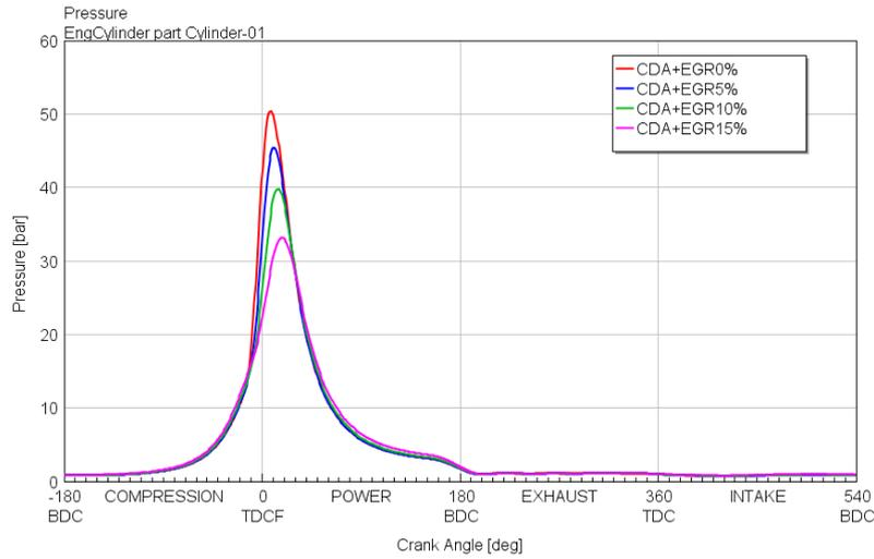
**Fig. 10 - In-cylinder pressure diagram for different percentage of EGR at 2000rpm@3bar BMEP**
