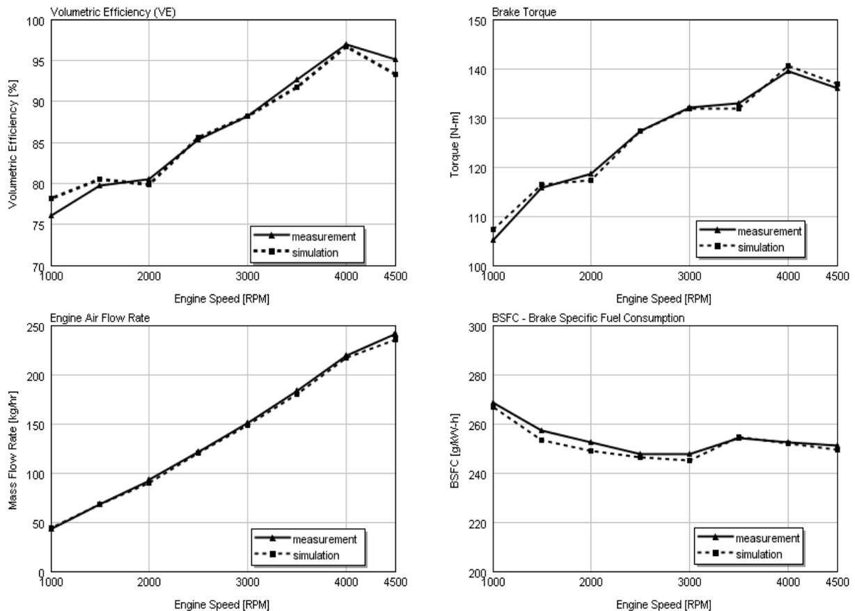
**Fig. 3 - Comparison between measured and simulated results at full load operations**
