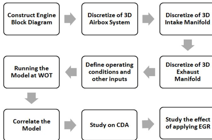
Fig. 1 - Steps of engine model construction
