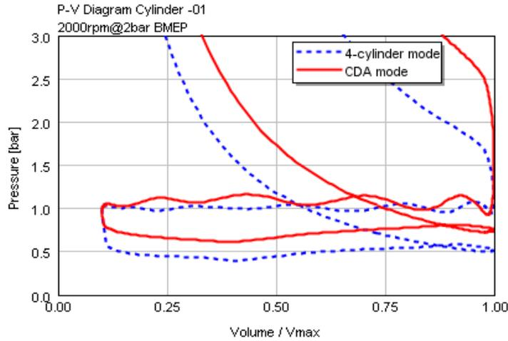
**Fig. 6 - Log P-V for cylinder 1 during normal 4-cylinder mode and CDA mode at 2000 rpm, 2 bar BMEP**
