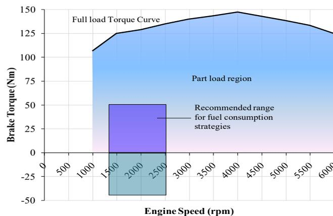
**Fig. 13 - Recommended brake torque range [11]**
