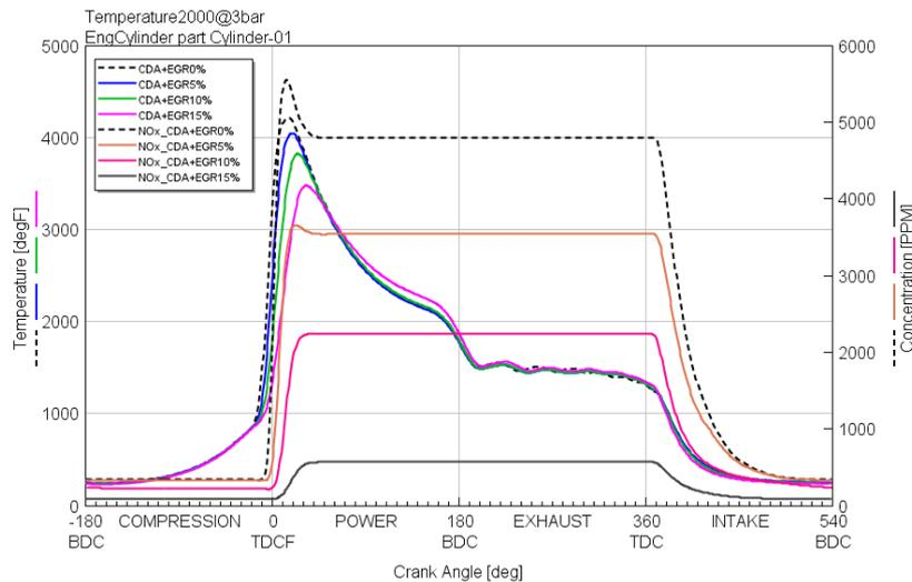
**Fig. 11 - In-cylinder combustion temperature and NO<sub>x</sub> formation for different percentage of EGR at 2000rpm@3bar BMEP**
