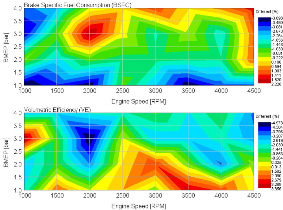
Fig. 4 - Percentage different between simulation and measurement data
