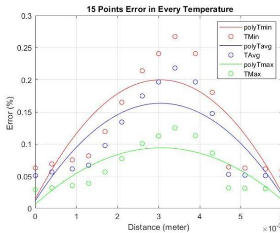
**Fig.- 7. Error in 15 points temperature distribution results with three ambient temperature conditions**
