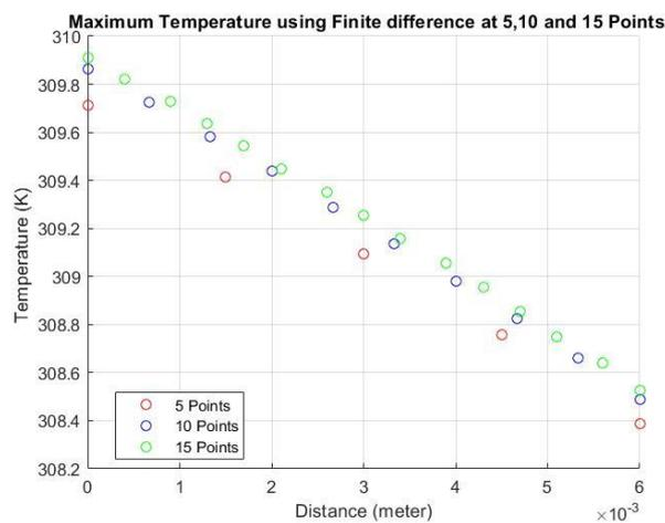
**Fig. -5 Relationship between 5, 10, and 15 points Distance to Temperature at Tmax temperature using the finite difference method**
