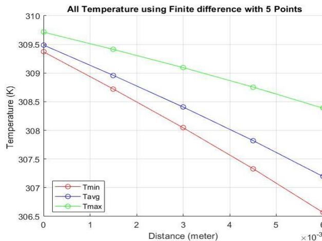
Fig.- 8. Graphic Relationship of the 5-point Distance to Temperature at 3 ambient temperature conditions
