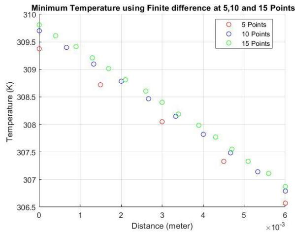
**Fig. 3- Relationship between 5, 10, and 15 points Distance to Temperature at Tmin temperature using the finite difference method**
