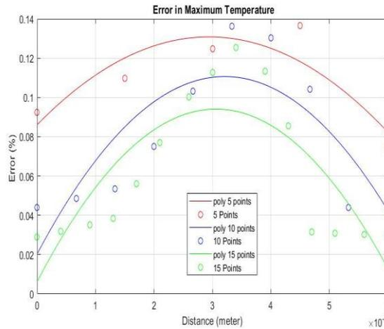
**Fig. -6. Error in 5,10 and 15 points temperature distribution results with the maximal ambient temperature**
