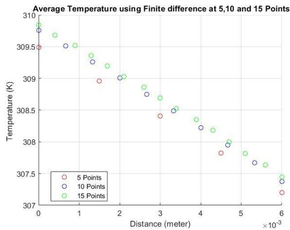
**Fig - 4 Relationship between 5, 10, and 15 points Distance to Temperature at Tavg temperature using the finite difference method**
