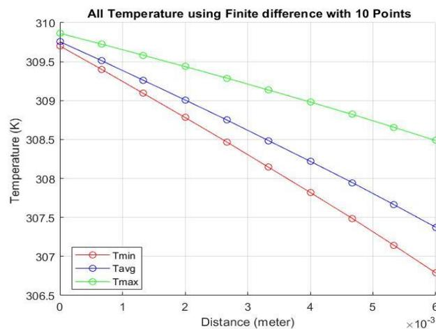
Fig.- 9. Graphic Relationship of 10-point Distance to Temperature at 3 ambient temperature conditions
