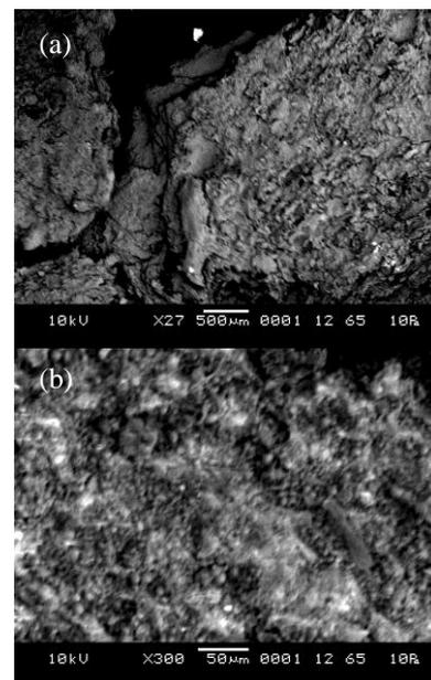
Fig.1 Scanning electron microscopy of cassava peel; a) and b) surface morphology of untreated cassava peel at x27 and x300 respectively
