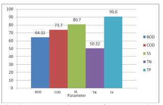
Fig. 12 Average removal percentage for parameter BOD, COD, SS, TN and TP
