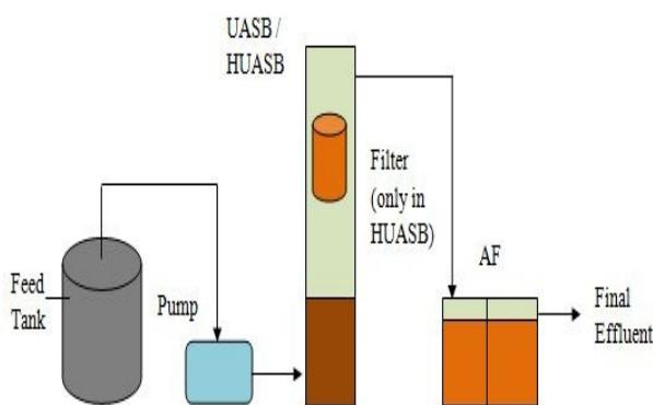
Fig. 1 Design for UASB-AF (R1) and HUASB-AF (R2) treatment system
