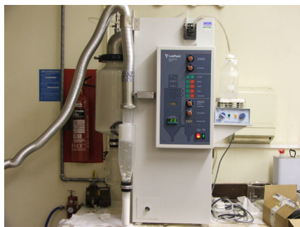
Fig. 3 SD-05 spray dryer machine used in production of powder
