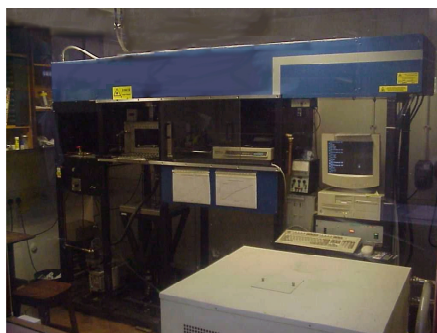
Fig. 4 CO 2 SLS experimental machine used to fabricate test specimen.
