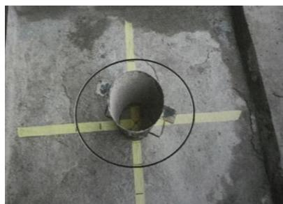
**Fig. 9 - Slump flow test**
