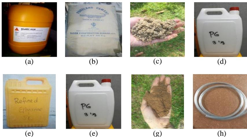
Fig. 3 - Materials in foamed concrete: (a) Foam agent, (b) Ordinary Portland Cement, (c) aggregate, (d) propylene glycol, (e) glycerin, (f) gypsum powder, (g) coconut shell powder, and (h) tube
