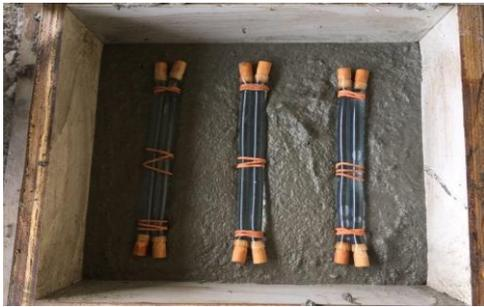
**Fig. 7 - The arrangement of the tube containing propylene glycol and glycerine**
