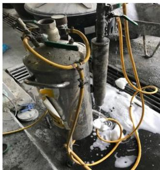
**Fig. 4 - Foaming agent mix by using an air compressor**
