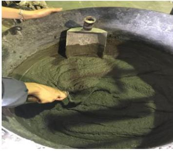
**Fig. 5 - Mixture of lightweight concrete**
