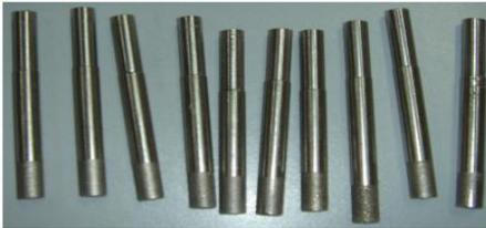
Figure 4: the machined tool steel using EDG processes
