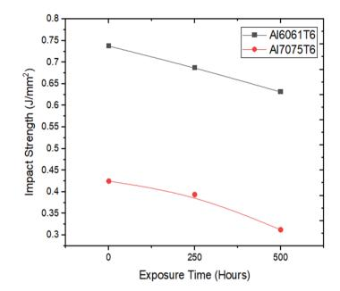
Fig. 9 - Variation of impact strength with exposure time
