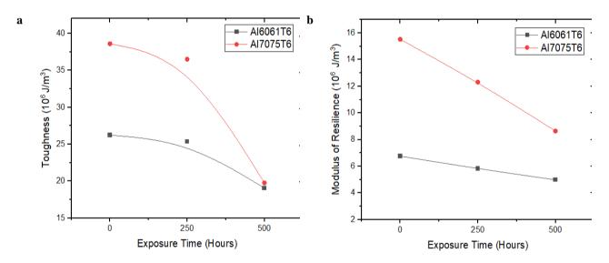
Fig. 7 - (a) Variation of Toughness with exposure time; (b) Variation of Elastic Resilience with exposure time
