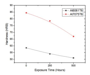
Fig. 8 - Variation of Rockwell Hardness Number (HRB) as a function of exposure time
