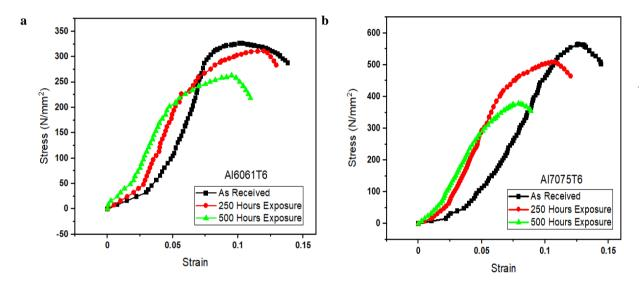
Fig. 3 - (a) Engineering stress-strain plot of (a) All6061T6; (b) Al7075T6
