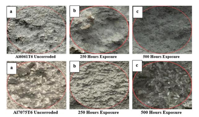
Fig. 11 - Optical surface images of fractured specimens representing with and without corrosion Al6061T6 and Al7075T6 (a) as-received samples (b) 250 hours; (c) 500 hours
