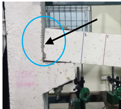
Fig. 7 - Uplift and crushing of CSCM specimen
