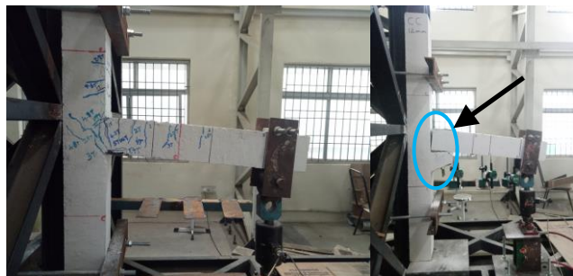
Fig. 4 -Tension cracks at the beam-column junction and lifting of beam in specimen
