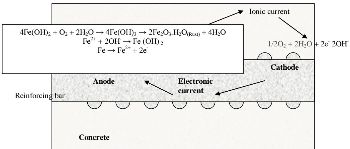
Fig.1 The corrosion reaction on steel.
