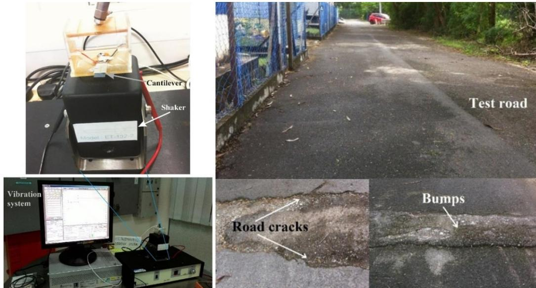
Fig. 3 - Experimental setup (Indoor and outdoor Test Road)
