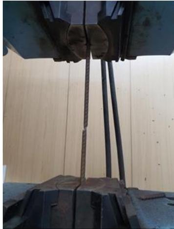
**Fig. 9 - The proposed 8 mm steel reinforcement tensile test at CEBL-Metal Lab**
