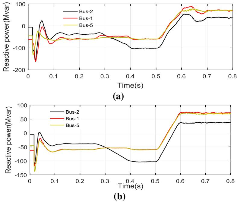
**Fig. 13 - Diagrams of reactive power flow results related to buses B1, B2, and B5 for two cases: using a) classic PI controller, and b) adaptive FL-PI controller**
