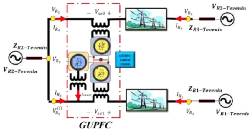
Fig. 1 - Model of a transmission line compensated by a GUPFC
