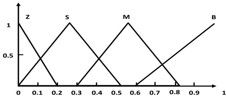
Fig. 8 - Membership function for the outputs  $K_p$  and  $K_i$
