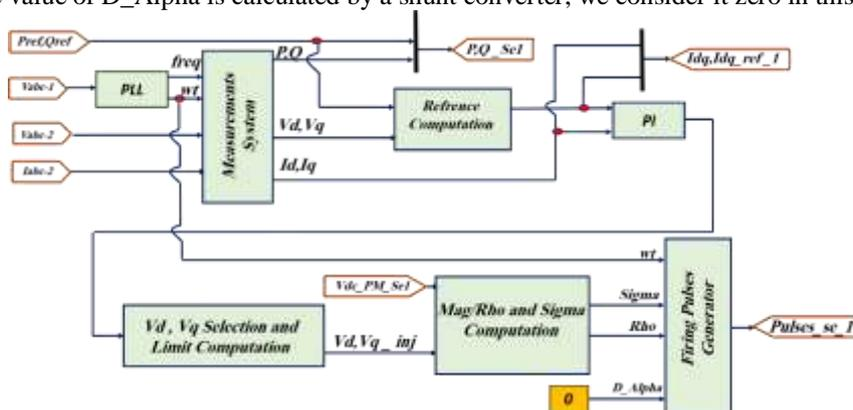
Fig. 3 - Series converter controller design for GUPFC compensator
