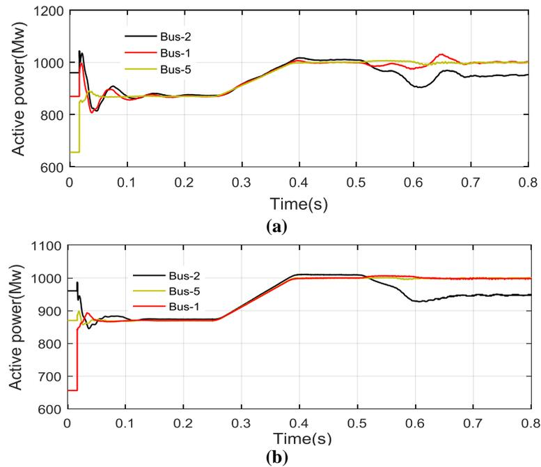
**Fig. 12 - Diagrams of active power flow results related to buses B1, B2, and B5 for two cases: using a) classic PI controller, and b) adaptive FL-PI controller**
