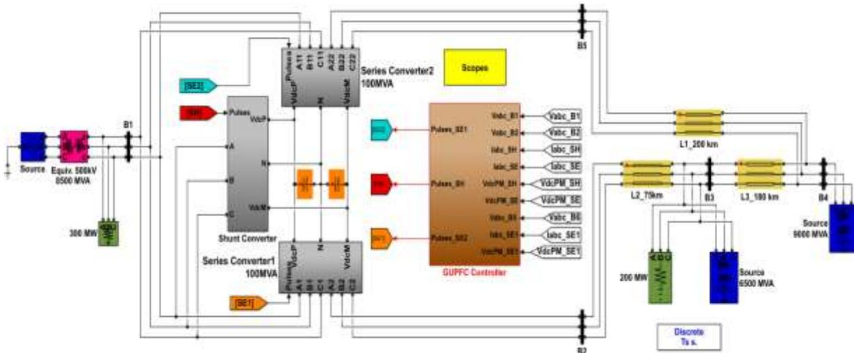
Fig. 9 - Simulation model of the 5-bus transmission network compensated by the GUPFC in MATLAB software
