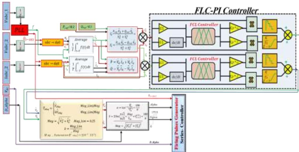
Fig. 5 - Control block diagram of the series converter 1 based on the FCL-PI control design
