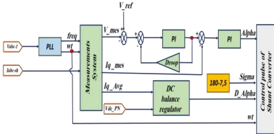
Fig. 2 - The control system of the GUPFC's shunt converter
