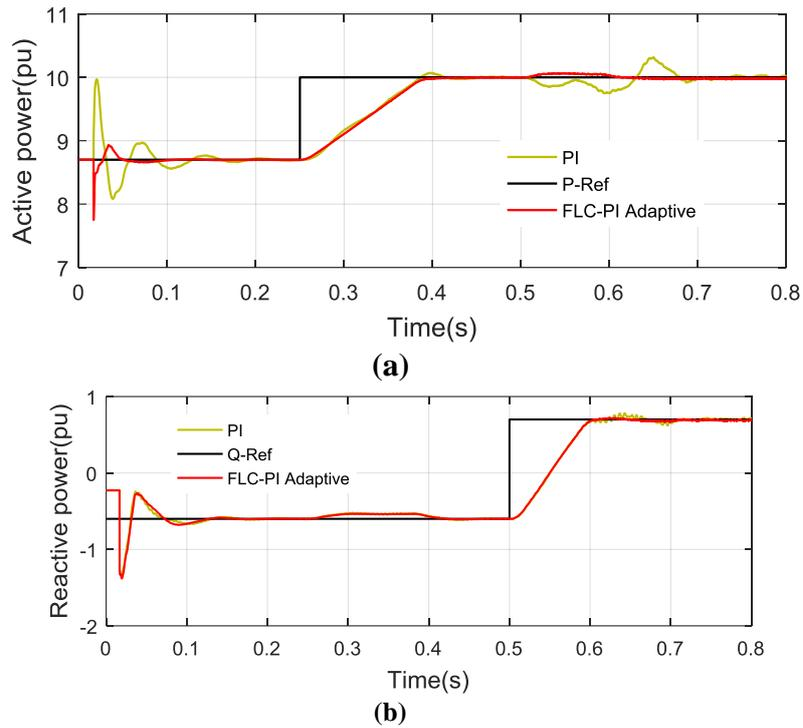
**Fig. 11 - Diagrams of a) active power, and b) reactive power tracking of series converter 2 using a PI controller and an FL-PI controller**
