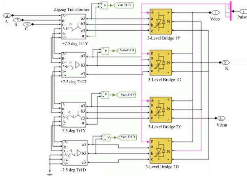
Fig. 4 - Model of the GUPFC's voltage source inverter for the shunt converter
