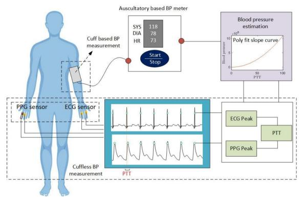
Fig. 1 - Proposed system architecture for blood pressure measurement system
