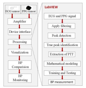
Fig. 5 - Measurement system flow diagram depicting blood pressure measurement
