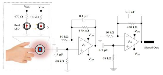
Fig. 3 - Bio signal conditioning circuit design
