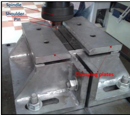
Fig. 1 - A photograph for the adaptive fixture to weld 2024 and 7075 Al alloys in a T-joint configuration.
