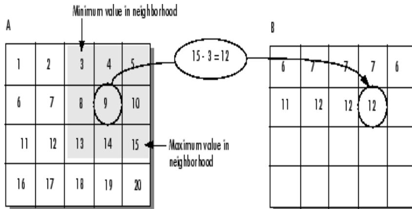
**Fig 4 - Examining values of pixel in range filtered output picture**
