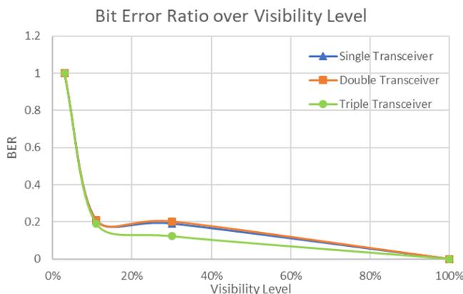
**Fig. 11 - Bit error ratio versus visibility level of transmission medium**
