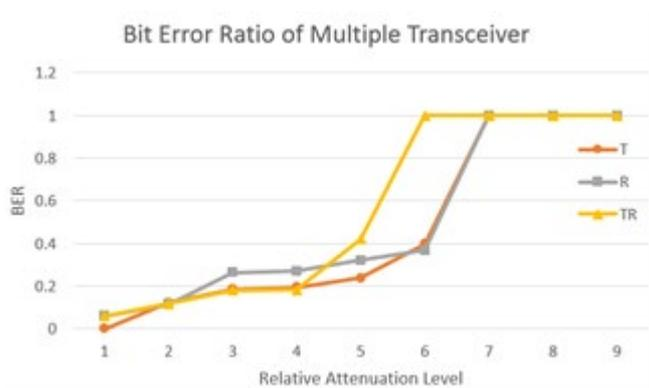
**Fig. 13 - Bit error ratio over attenuation level under the modeled turbulence**
