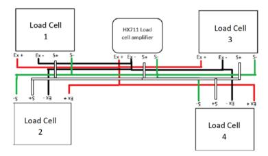
Fig. 5 - Circuit diagrams for S-type TAS501 load cells
