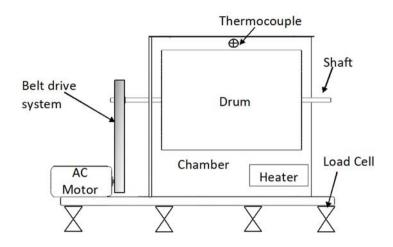
Fig. 3 - Schematic diagram for rotary drum dryer
