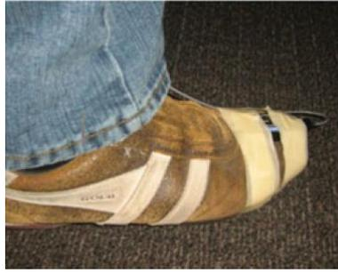
**Fig. 1 - Inertial sensor attached to a shoe**
