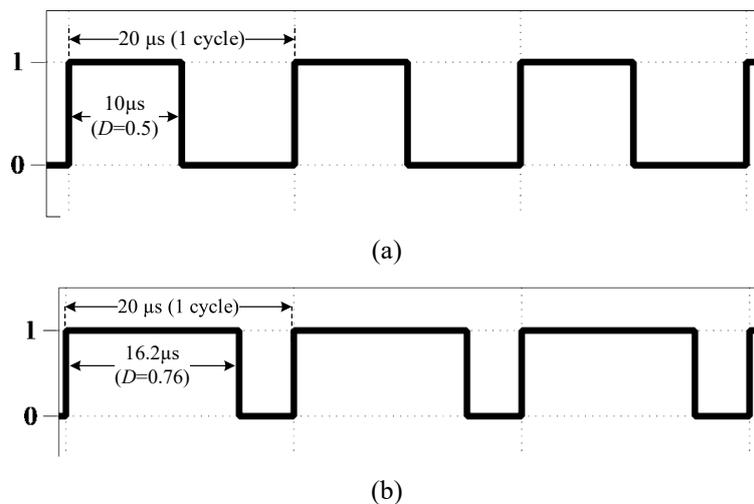
Fig. 4 - CDBC switching scheme for (a) 0.5 duty cycle (b) 0.76 duty cycle
