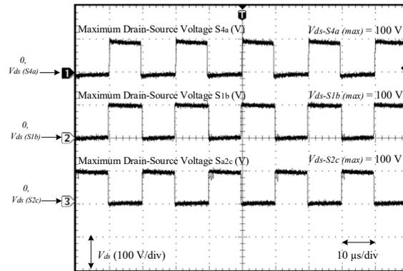
Fig. 12 - Experiment result of 4-level SMMC voltage stress at 0.5 duty cycle with  $V_{in} = 48V$
