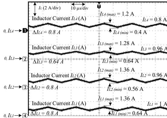
Fig. 10 - Experiment result for input inductor current stress of 4-level SMMC
