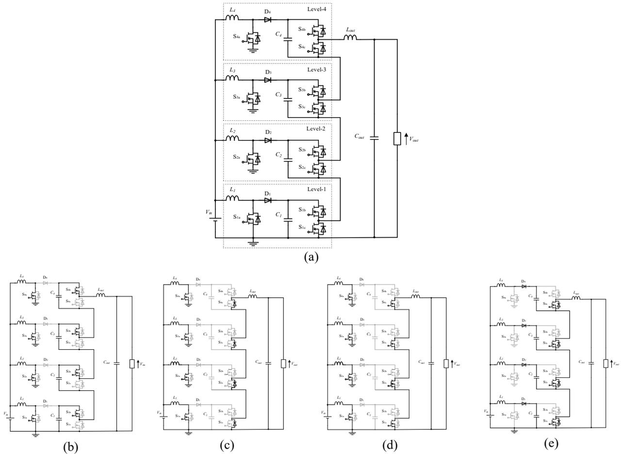
**Fig. 5 - Circuit structure of 4-level SMMC (a) Main circuit structure (b) Mode 1: Capacitor discharging in series (c) Mode 2: Dead-time (d) Mode 3: Time-delayed (e) Mode 4: Capacitor charging in parallel**
