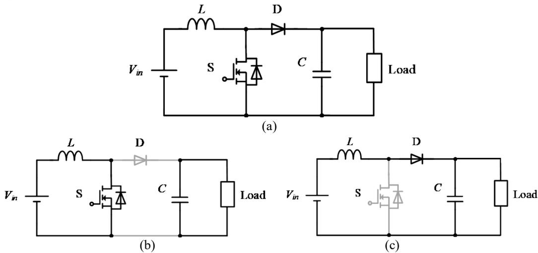
Fig. 3 - Circuit structure of CDBC (a) Main circuit structure (b) Operation mode 1 (c) Operation mode 2
