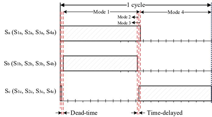
**Fig. 6 - 4-level SMMC switching scheme**
