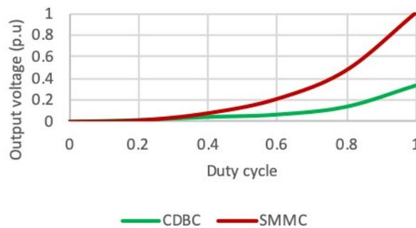
Fig. 2 - Relationship of duty cycle against output voltage (p.u.) for CDBC and SMMC
