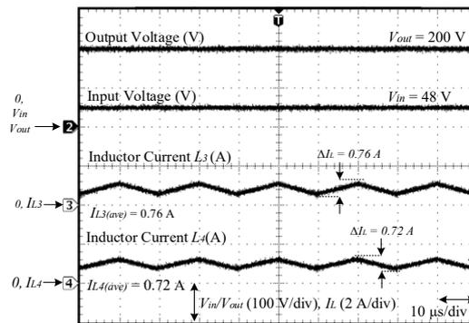
Fig. 8 - Experimental result of 4-level SMMC for  $D = 0.5$
