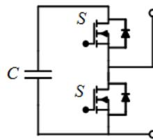
Fig. 1 - Marx topology modular block principle
