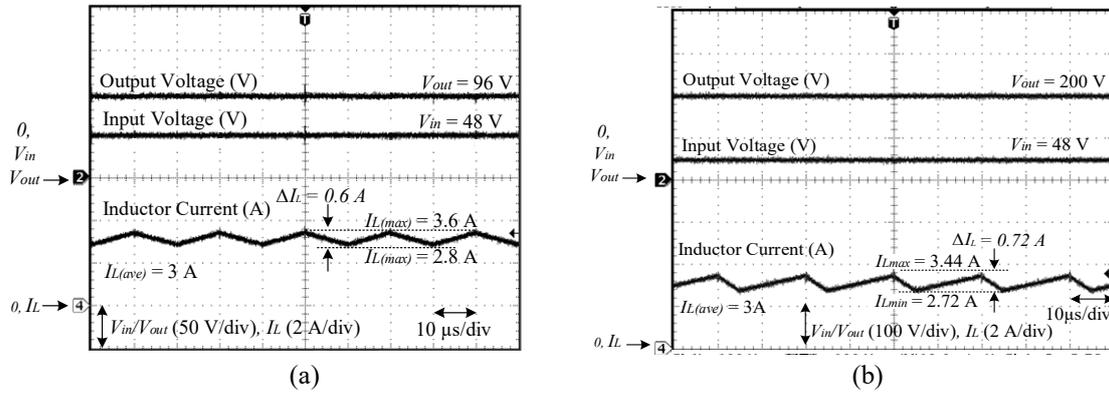
Fig. 7 - Experimental results of CDCC when (a)  $D = 0.5$ , and (b)  $D = 0.76$
