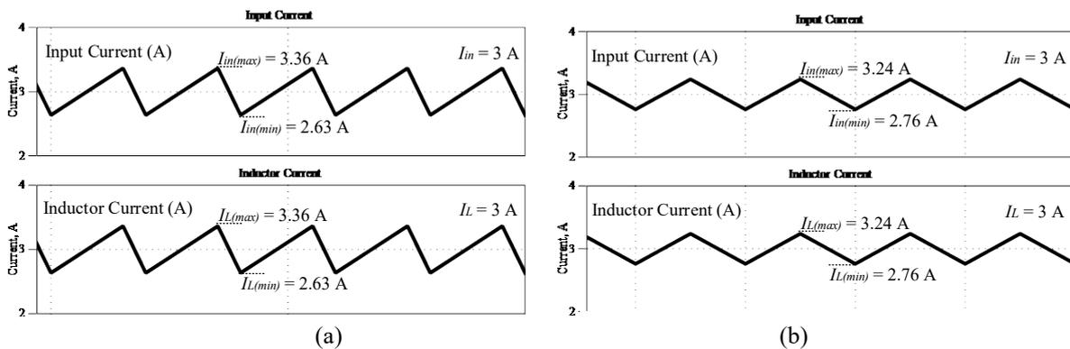
Fig. 9 - Simulation results of current stress on input inductor of CDCC at  $L_{in} = 1 \text{ mH}$  for (a) at 0.5 duty cycle and (b) at 0.76 duty cycle.
