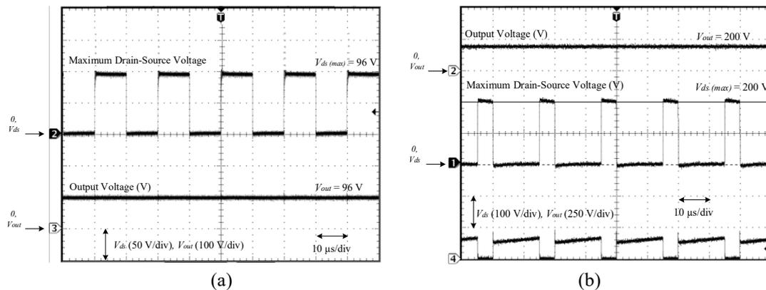
Fig. 11 - Experiment results of CDBC voltage stress with  $V_{in} = 48V$  (a) at 0.5 duty cycle,  $V_{out} = 96 V$  (b) at 0.76 duty cycle,  $V_{out} = 200 V$
