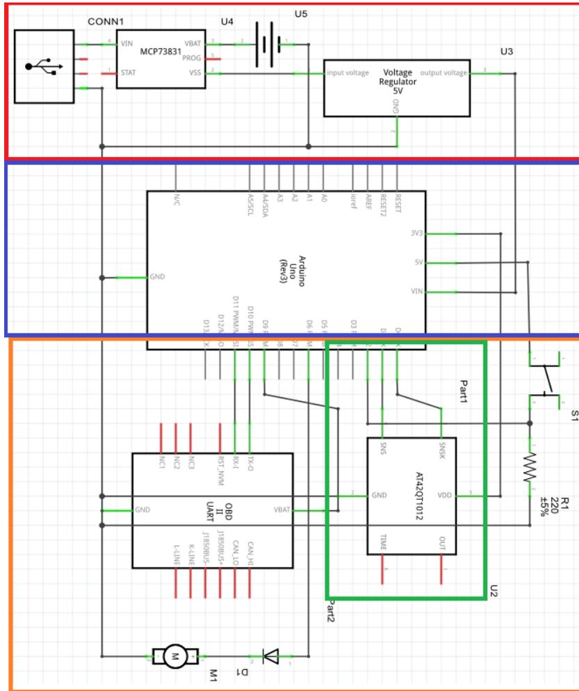
Fig. 5 - Schematic diagram on wirings of the lock unit
