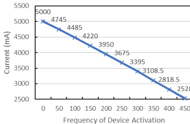
Fig. 8 - Battery life cycle per full charge
