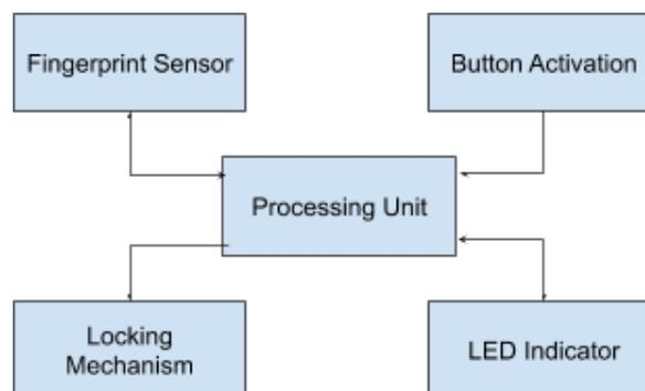
**Fig. 3 - Interactions of components in the lock system**
