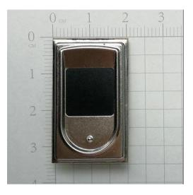
Fig. 2 - R300 UART Fingerprint Reader
