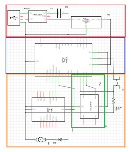
Fig. 5 - Schematic diagram on wirings of the lock unit
