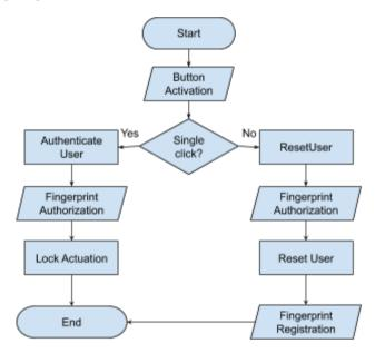
Fig. 4 - Process flowchart of lock functions
