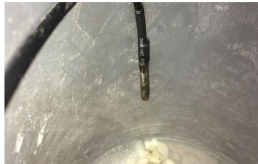
**Fig. 7 - Attachment of the temperature sensor**
