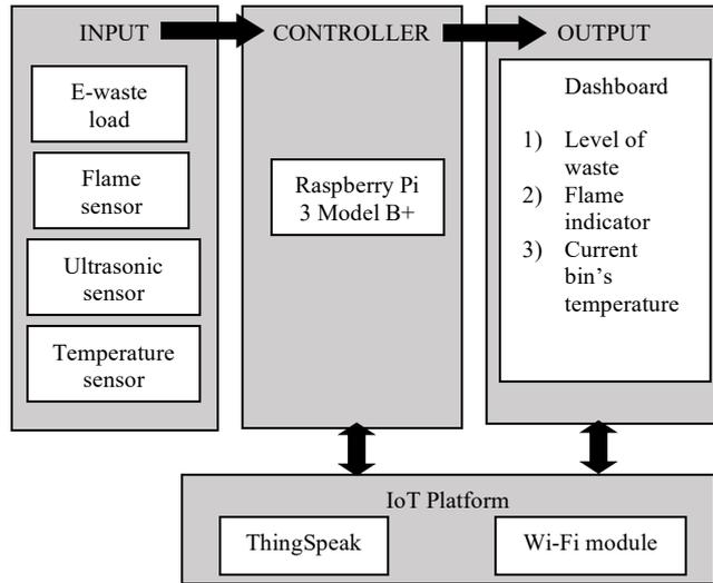
**Fig. 2 - IoT E-waste monitoring system block diagram**
