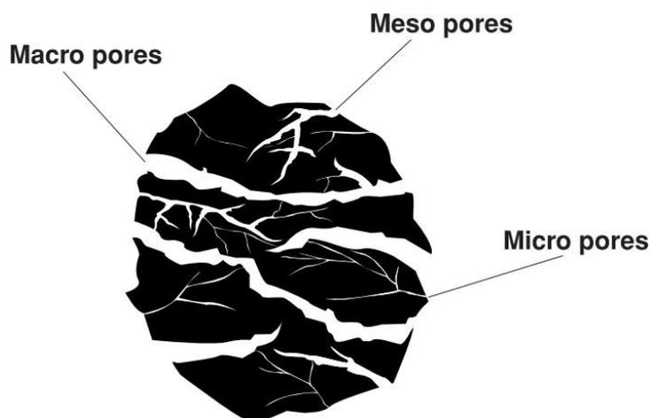
Fig. 2 - Pores of activated carbon [39]
