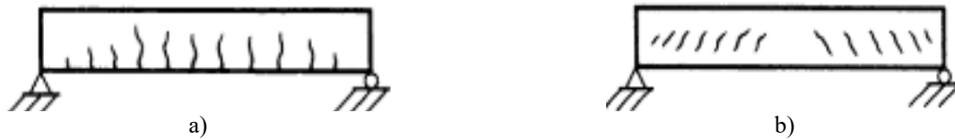
Fig. 5 - (a) Crack pattern due to bending force, (b) Crack patterns due to shear force
