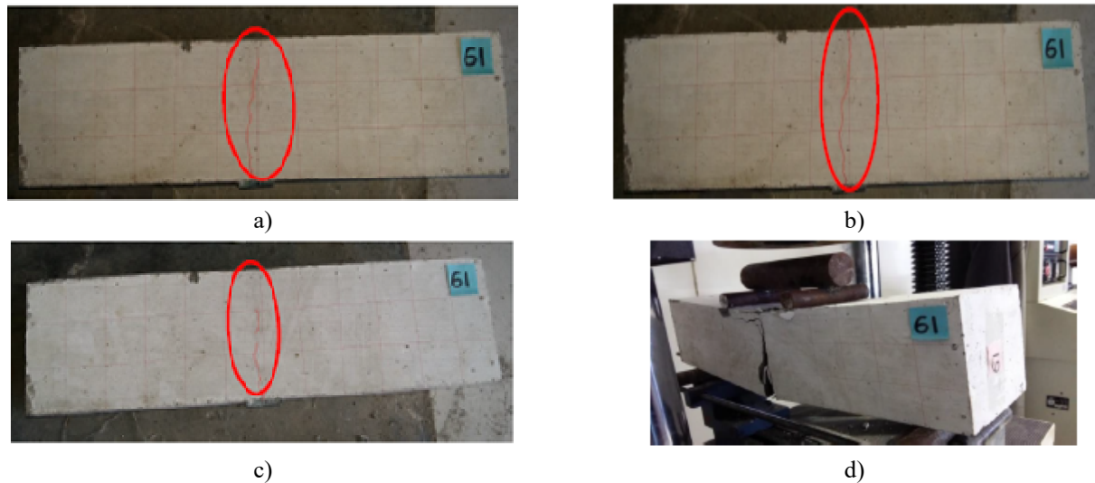
Fig. 12 – (a) Cracks that have been injected by bacteria for 14 days, (b) Cracks that have been injected by bacteria for 21 days, (c) Cracks that have been injected by bacteria for 28 days, (d) Flexural failure on the beam after repair
