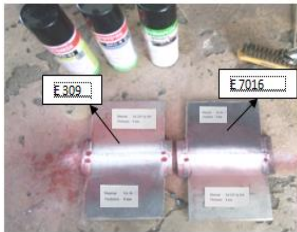
Fig. 3 - NDT Penetrant method of a solvent removable system for both samples with differences of the electrode
