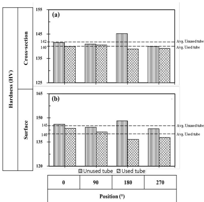
Fig. 8 - Results from hardness test of unused and used tube (a) Cross-section; (b) surface
