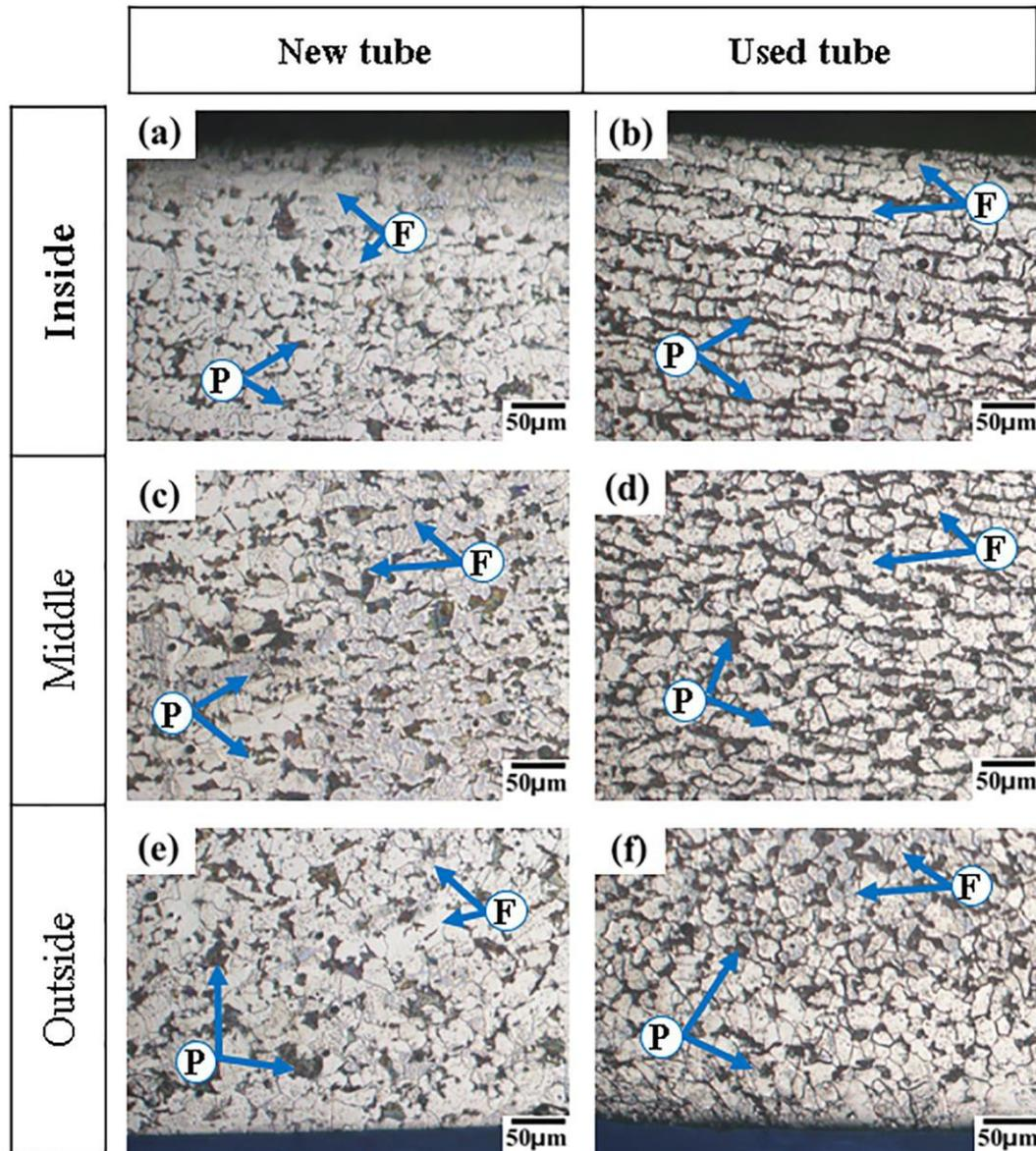
**Fig. 5 - Representative optical micrographs of (a-b) inside of the unused and used tube, (c-d) mid-wall of the unused tube and used tube; (e-f) outside of the unused tube and used tube exhibiting black regions of pearlite (P) and white regions of ferrite ( F )**
