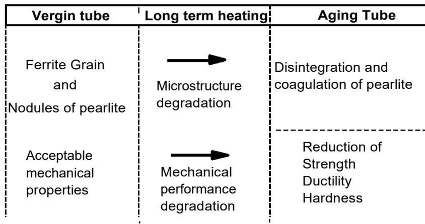
**Fig. 9 - The schematic diagram in elucidating the microstructure and mechanical degradation of SA210 A1 steel subjected to an actual boiler environment**
