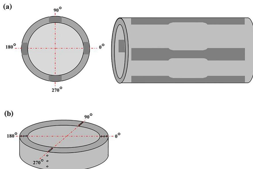
**Fig. 1 - (a) positions of the tensile specimen preparation; (b) positions of the hardness measurement**
