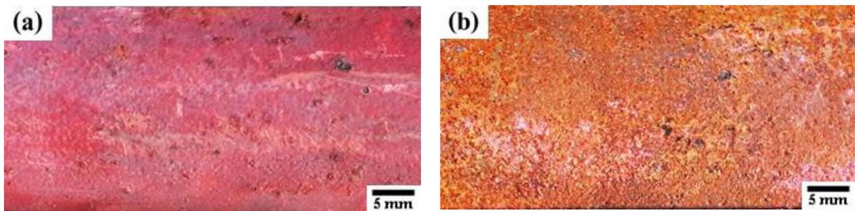
**Fig. 3 - Outer surface conditions (a) the unused tube; (b) used tube**
