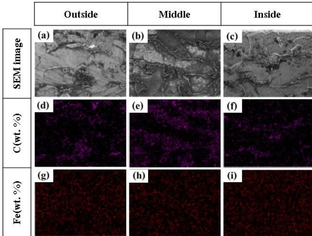
**Fig.6 - SEM micrograph together with EDS analysis of used steel tube (50X) of outside, mid-wall, and inside of the used tube (a -c) SEM image, (d-f) Distribution of carbon; (g-f) Distribution of ferrous**
