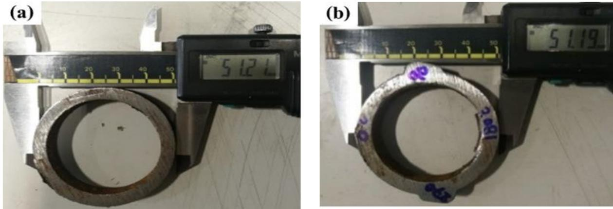
**Fig. 2 - The dimension check at the outside diameter (a) unused tube; (b) used tube**
