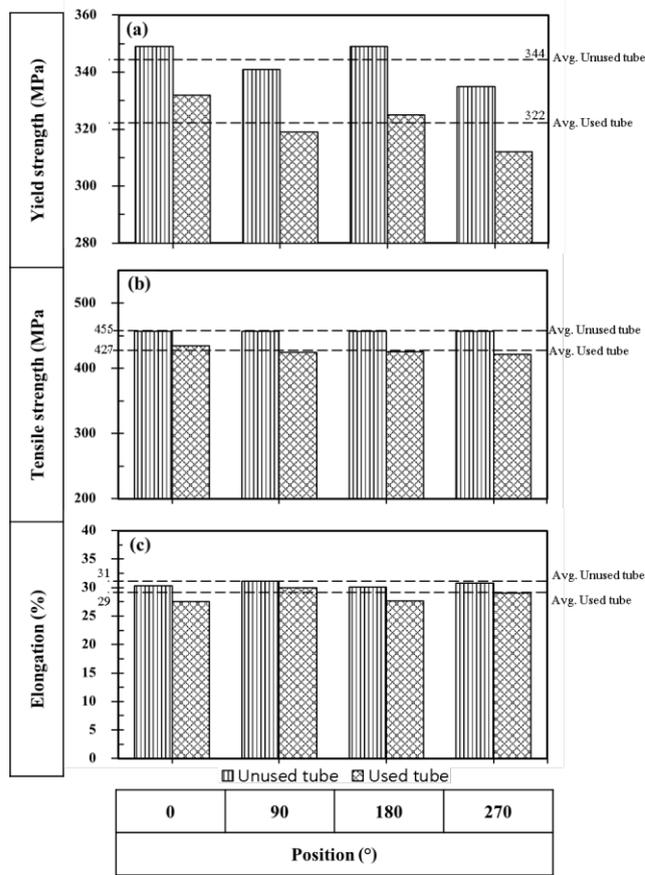
Fig. 7 - Results from tensile test of unused and used tube (a) yield strength, (b) tensile strength; (c) elongation
