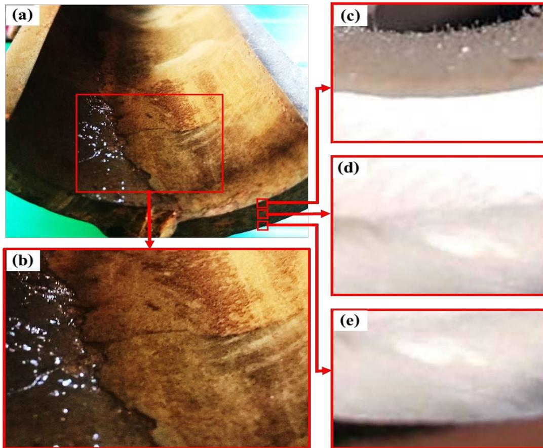
**Fig. 4 - Visual inspection for inner surface conditions of the used tube (a) inner surface; (b-e) high magnification views of inner surface**
