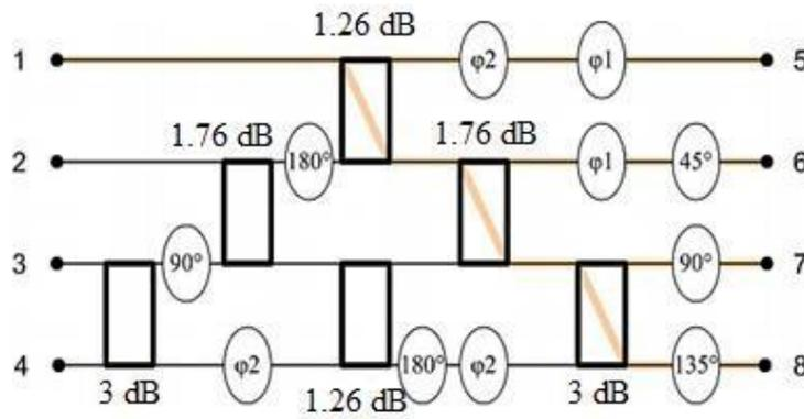
**Fig. 8 - Block diagram of the proposed 4 x 4 Nolen Matrix based on coupler delay compensation of broadband substrate integrated waveguide (SIW) [16]**
