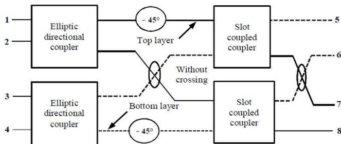
**Fig. 5 – Block diagram of the two layers wideband 4 x 4 Butler matrix [21]**
