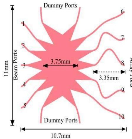
Fig. 1 - Layout design of Rotman lens geometry [4]
