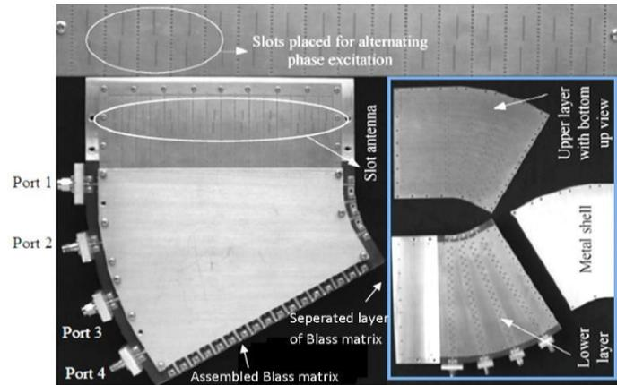
**Fig. 6 - Photograph of the proposed SIW planar 4 × 16 Blass matrix [24]**
