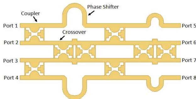
**Fig. 4 - Layout of the proposed 4 x 4 miniaturized Butler matrix beamforming network [20]**
