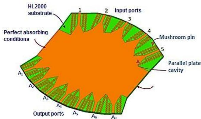
Fig. 2 - Ideal model of Rotman lens with ridge gap waveguides (RGW) [5]
