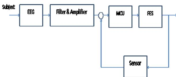
Figure 3: BCI-FES Control Scheme System
