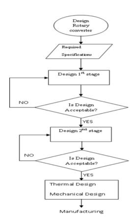
Fig.4. General Flow chart layout explains sequential steps of design rotary converter electric machine.
