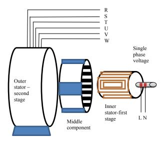
Fig.5. General Shape of six – phase rotary converter machine.
