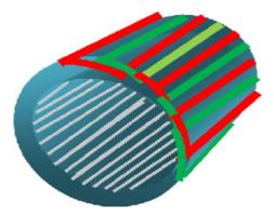
Fig.2. Component 2, Dual functions, the inside surface as armature of single phase I.M. and in same time the outside surface as a stator of synchronism R.C.
