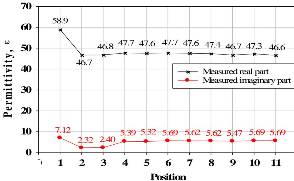
**Fig. 4 - Measured value of real part,  $\epsilon'$  (re) and the imaginary part,  $\epsilon''$  (im) of permittivity on the bottom surface of skin phantom**
