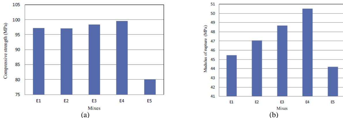
**Fig. 6 - a) The effect of fine-sand ratio on the adhesive cubes compressive strength, b) The effect of fine-sand ratio to the modulus of rupture of adhesive the prisms [61]**
