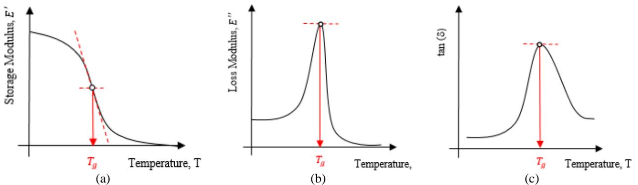
**Fig. 2 - Schematic representation of several key temperature values during glass transition [25]**
