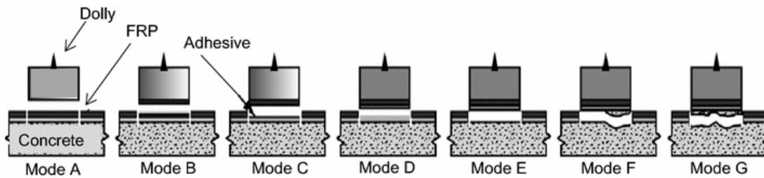
Fig. 4 - Failure modes for the pull of test [61]
