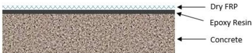
Fig.1 - Step by step installation by wet lay-up technique
