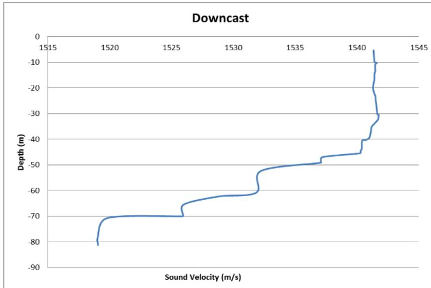
Fig. 9 - The sound velocity profile during downcast at Lat: 06° 36' N, Long: 098° 57' 46.05" E
