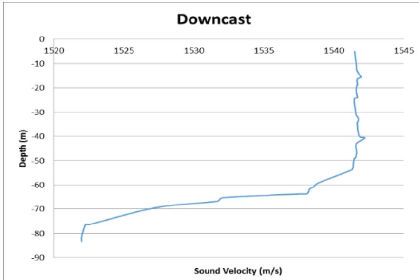
**Fig. 5 - The sound velocity profile during downcast at Lat: 05° 52.54’ N, Long: 098° 26.38’ E**
