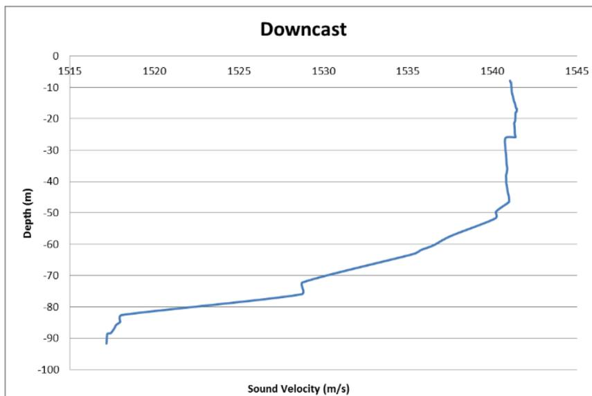
Fig. 13 - The sound velocity profile during downcast at Lat: 06° 06' 34.33" N, Long: 098° 28' 11.08" E
