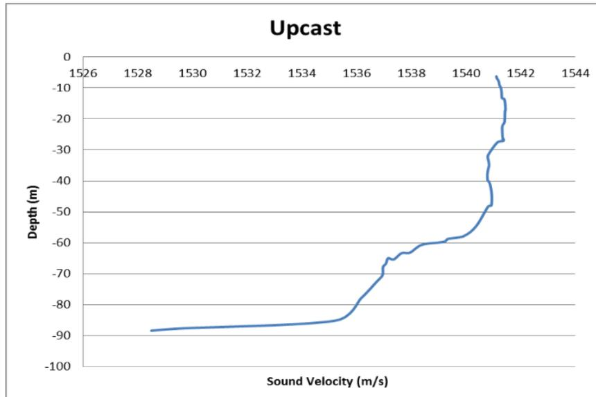
Fig. 14 - The sound velocity profile during upcast at Lat: 06° 06' 34.33" N, Long: 098° 28' 11.08" E
