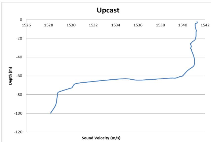
Fig. 20 -The sound velocity during upcast at Lat: 06° 11' 56.93" N, Long: 098° 42' 21.36" E
