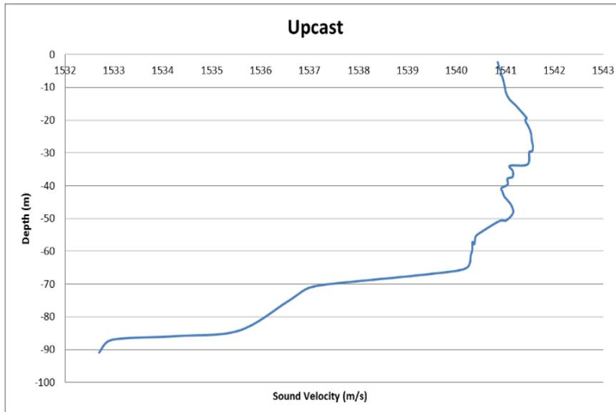
Fig. 18 -The sound velocity during upcast at Lat: 05° 59' 36.93" N, Long: 098° 37' 21.36" E
