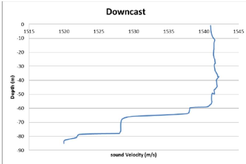
**Fig. 3 - The sound velocity profile during downcast at Lat: 05° 53.55'N, Long: 098° 30.46' E**
