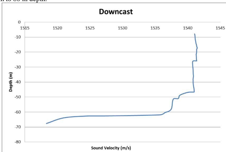
Fig. 15 - The sound velocity profile during downcast at Lat: 05° 57' 49.6" N, Long: 098° 37' 12.75" E
