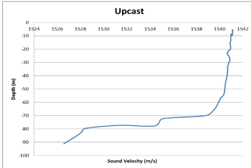
Fig. 12 - The sound velocity profile during upcast at Lat: 06° 05' 34.33" N, Long: 098° 27' 37.08" E
