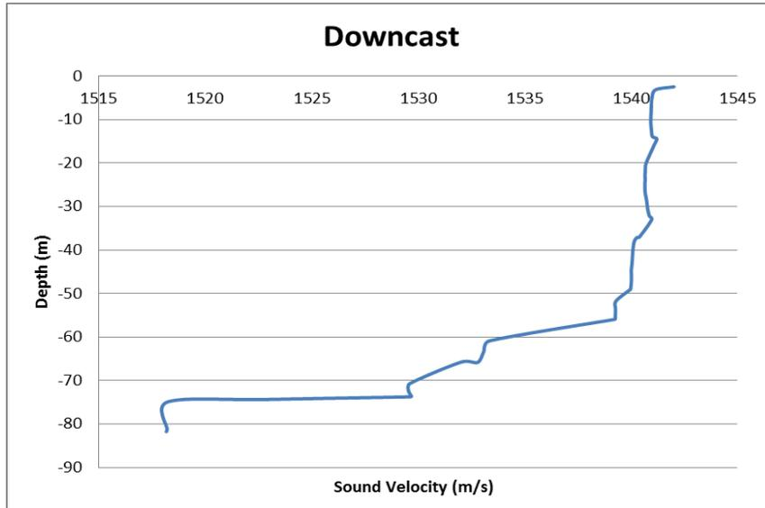
**Fig. 7 - The sound velocity profile during downcast at Lat: 06° 04.32' N, Long: 098° 26.38' E**
