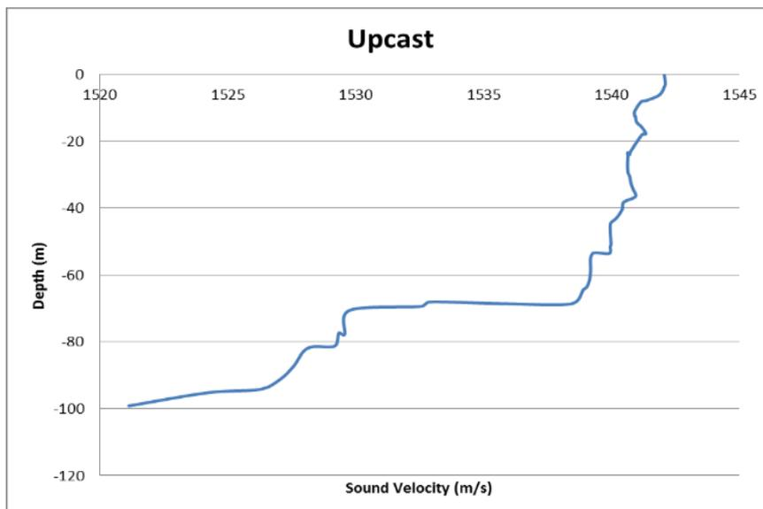
**Fig. 8 - The sound velocity profile during upcast at Lat: 06° 04.32' N, Long: 098° 26.38' E**
