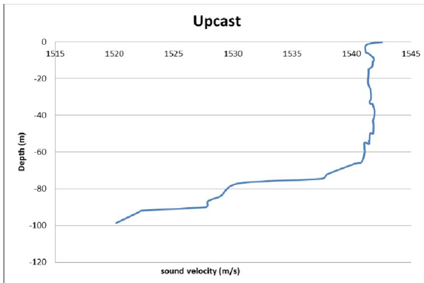
**Fig. 4 - The sound velocity profile during upcast at Lat: 05° 53.55'N, Long: 098° 30.46' E**
