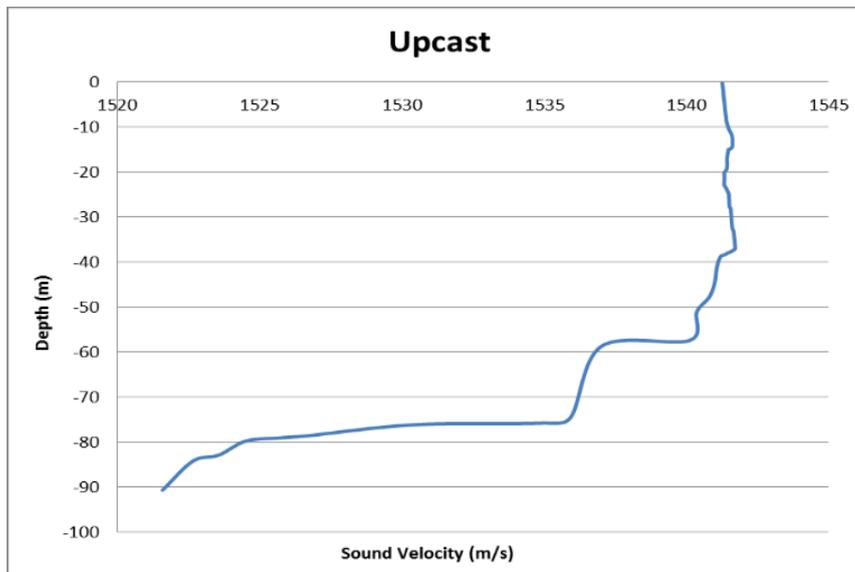
Fig. 10 - The sound velocity profile during upcast at Lat: 06° 36' N, Long: 098° 57' 46.05" E
