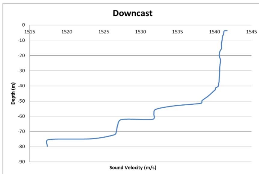
Fig. 11 - The sound velocity profile during downcast at Lat: 06° 05' 34.33" N, Long: 098° 27' 37.08" E
