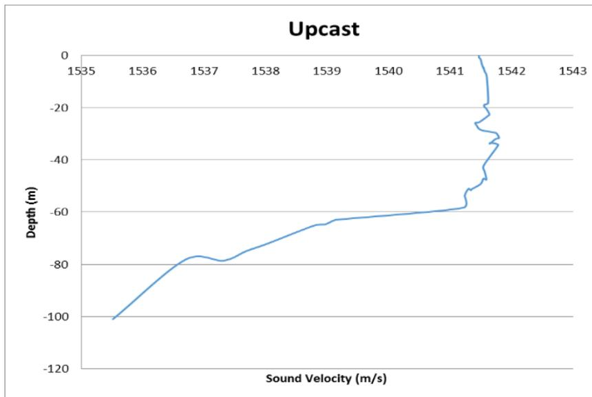
**Fig. 6 - The sound velocity profile during upcast at Lat: 05° 52.54’ N, Long: 098° 26.38’ E**
