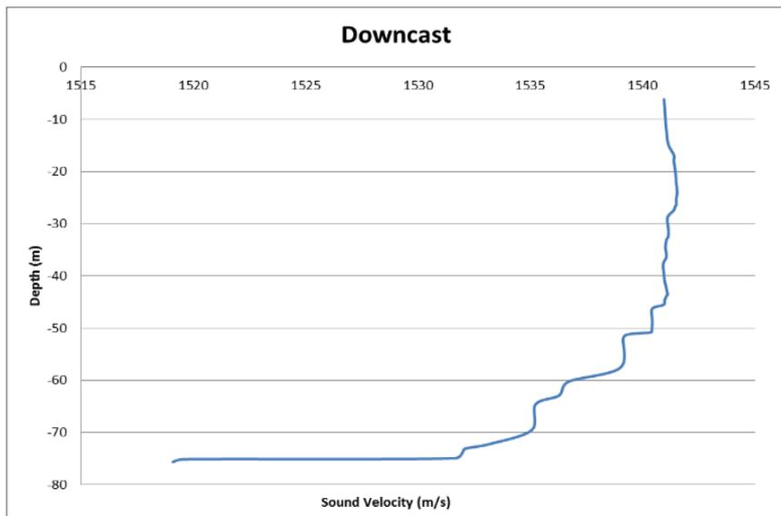
Fig. 17 - The sound velocity profile during downcast at Lat: 05° 59'36.93" N, Long: 098° 37' 21.36"E
