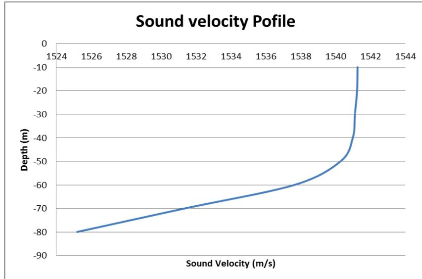
Fig. 21 - The average sound velocity profile for overall location at every 10 m depth
