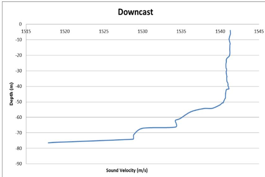
Fig. 19 -The sound velocity during downcast at Lat: 06° 11' 56.93" N, Long: 098° 42' 21.36" E
