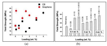
Fig. 4 - (a) Yield strength values for epoxy composite containing individual CB and graphene fillers; (b) yield strength values for epoxy composite containing dual fillers, with single filler also shown for comparison
