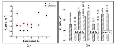
Fig. 2 - (a) K<sub>IC</sub> values for epoxy composite containing individual CB and graphene fillers and (b) K<sub>IC</sub> values for epoxy composite containing dual fillers, with single filler also shown for comparison
