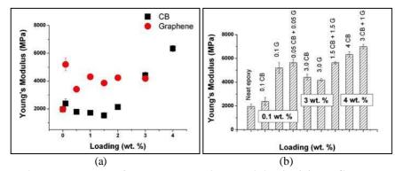
Fig. 3 - (a)Young's Modulus values for epoxy composite containing individual CB and graphene fillers; (b)Young's Modulus values for epoxy composite containing dual fillers, with single filler also shown for comparison
