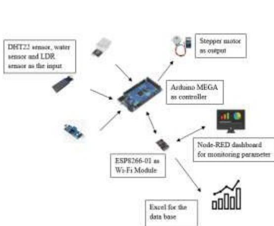
Fig. 4 - Aquaponics design structure
