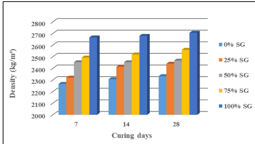
Fig. 4 - Density of mortar against curing periods
