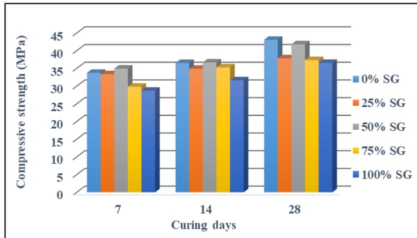
Fig. 6 - Compressive strength against curing periods
