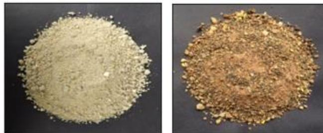
**Fig. 1 - Fine aggregates used (a) River sand and (b) spent garnet**
