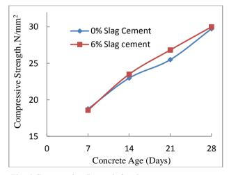
Fig. 4 Compressive Strength for slag aggregate concrete (SAC) with 6% slag cementitious replacement.
