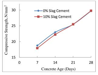
Fig.6: Compressive strength for slag aggregate concrete (SAC) with 10% slag cementitious replacement.
