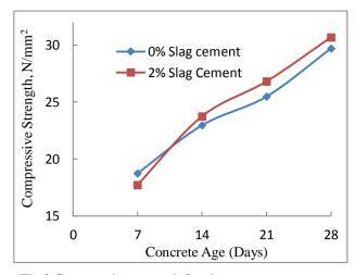
Fig 2 Compressive strength for slag aggregate concrete (SAC) with 2% slag cementitious replacement.
