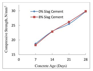
Fig. 5 Compressive strength for slag aggregate concrete (SAC) with 8% slag cementitious replacement.
