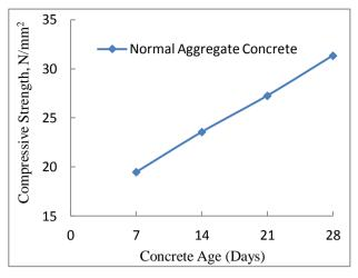
Fig. 1 Compressive strength for normal aggregate concrete (NAC) with 100% ordinary Portland cement.
