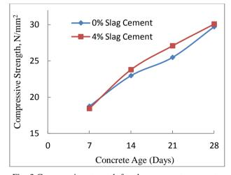
Fig. 3 Compressive strength for slag aggregate concrete (SAC) with 4% slag cementitious replacement.
