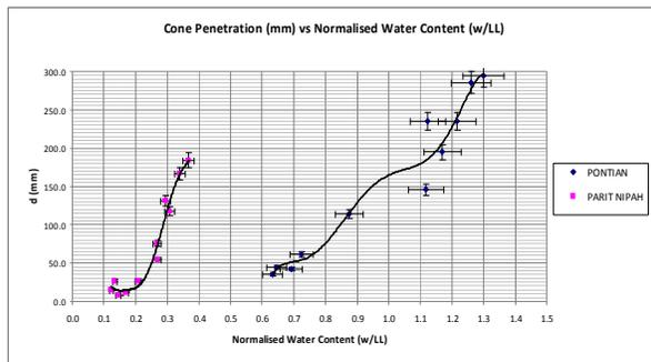
Fig. 13 Graph Depth of Cone Penetration versus Normalised water content for Parit Nipah Peat and Pontian Peat
