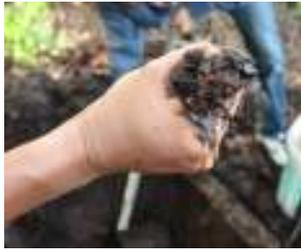
Fig. 6. Von Post Squeezing Test
