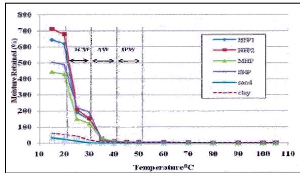
Fig. 10 Comparison of moisture content loss for different samples.
