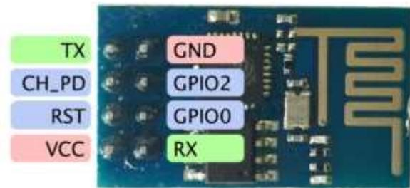
Fig. 12 - Hardware structure of ESP-8266
