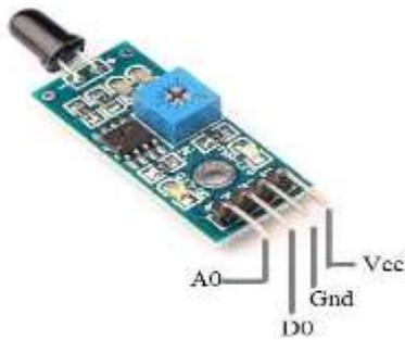
Fig. 11 - Hardware structure of flame sensor
