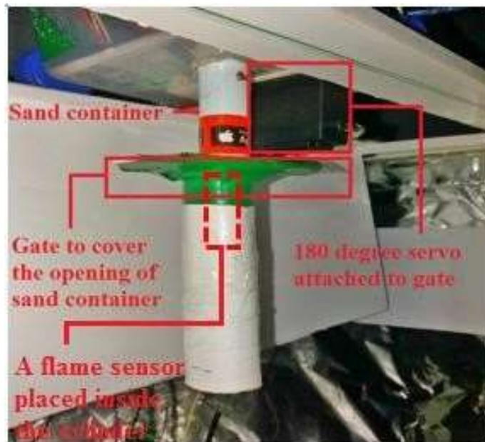
Fig. 8 - Sand-Pouring Mechanism
