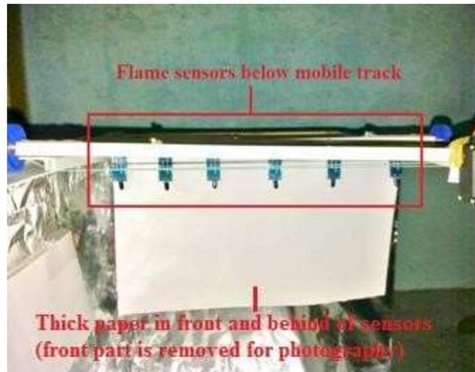
**Fig. 9 - an array of flame sensor mechanism**
