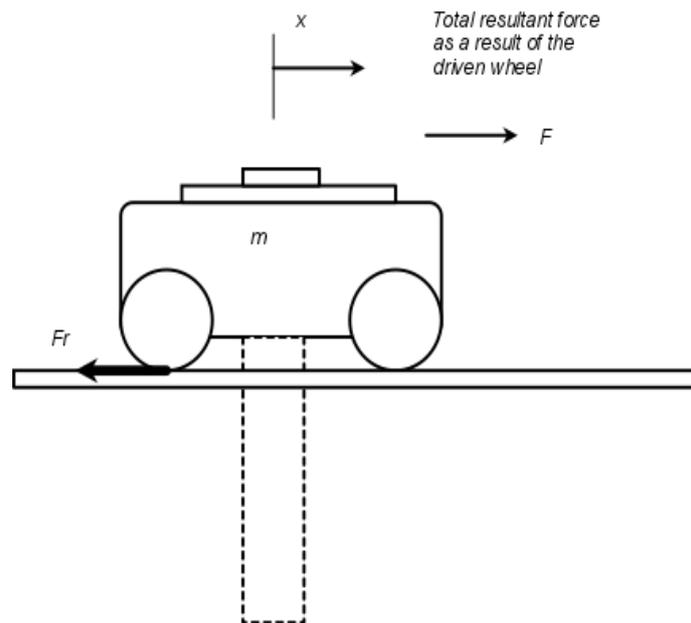
Fig. 3 - Free body diagram representing fire fighter robot
