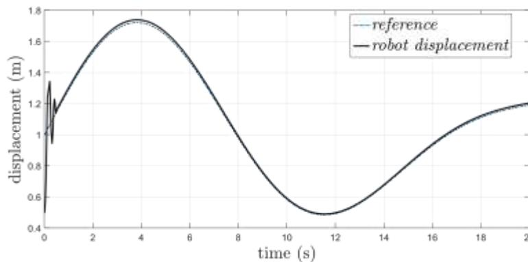
**Fig. 4 - Displacement of the fire fighter robot following a desired trajectory emulating the soft movement of the robot to avoid sand spillage**
