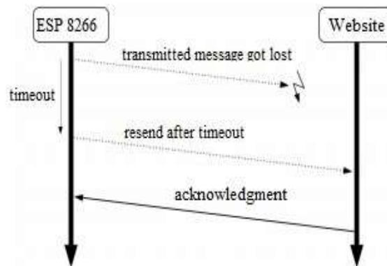
Fig. 13 - Communication protocol between ESP 8266 application layer with the target website
