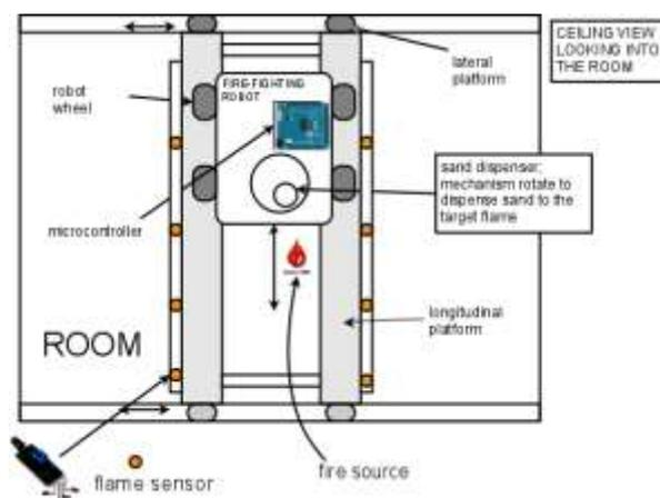
Fig. 1 - Fire detection and extinguishing method illustration
