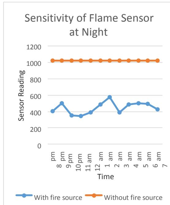
Fig. 15 - Sensitivity of flame sensor at night
