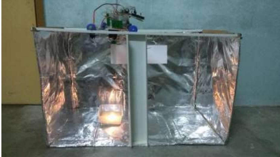
**Fig. 17 - Fire Fighter Robot moved to fire source to pour down sand**
