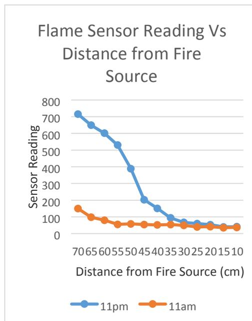
Fig. 16 - Flame sensor reading at 11pm and 11am versus distance from fire source
