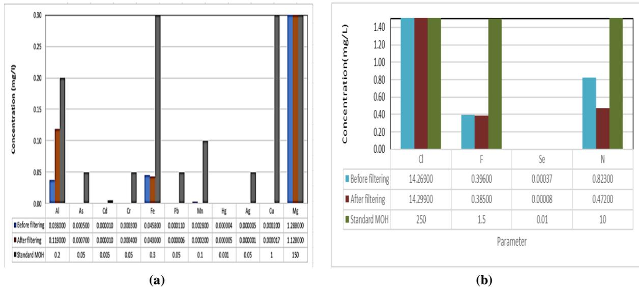
**Fig. 4 - (a) The cation heavy metals concentrations of water before and after through water filter system by brand U (Model 1), and (b) The anion heavy metals concentrations of water before and after through water filter system by brand U (Model 1)**
